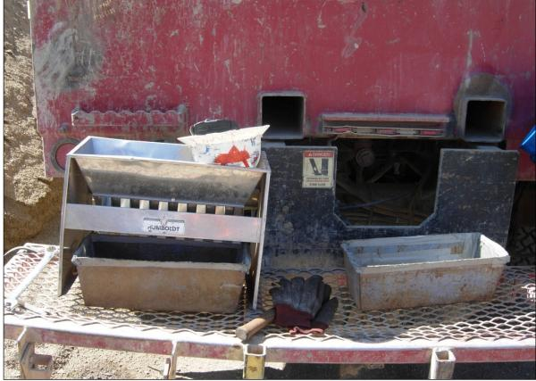
Source: SRK, 2018 Figure 10-8: Riffle Splitter Used at Drill Site
