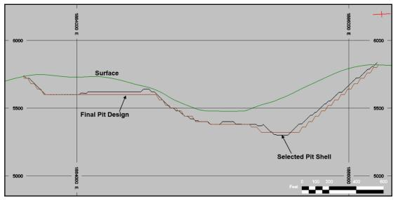
Figure 16-5: Section 2 Showing Mine Design and Selected Pit Shell
