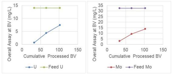
Figure 13-4: Uranium and Molybdenum Removal by Ion Exchange on Purolite A660 Resin
