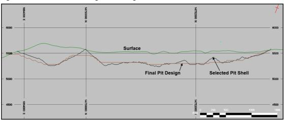
Figure 16-4: Section 1 Showing Mine Design and Selected Pit Shell
