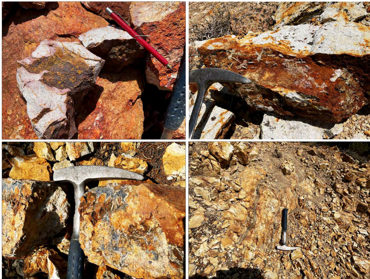
Figure 5. Strongly altered and mineralized, finely porphyritic House Canyon rhyolite from the King Solomon mine area. Dense, finely porphyritic plagioclase-biotite-quartz rhyolite is pervasively sericitized and moderately silicified. Jarosite (upper left), barite (upper right), stibnite (lower photographs) are common features of the Au-Ag-Sb mineralization.
