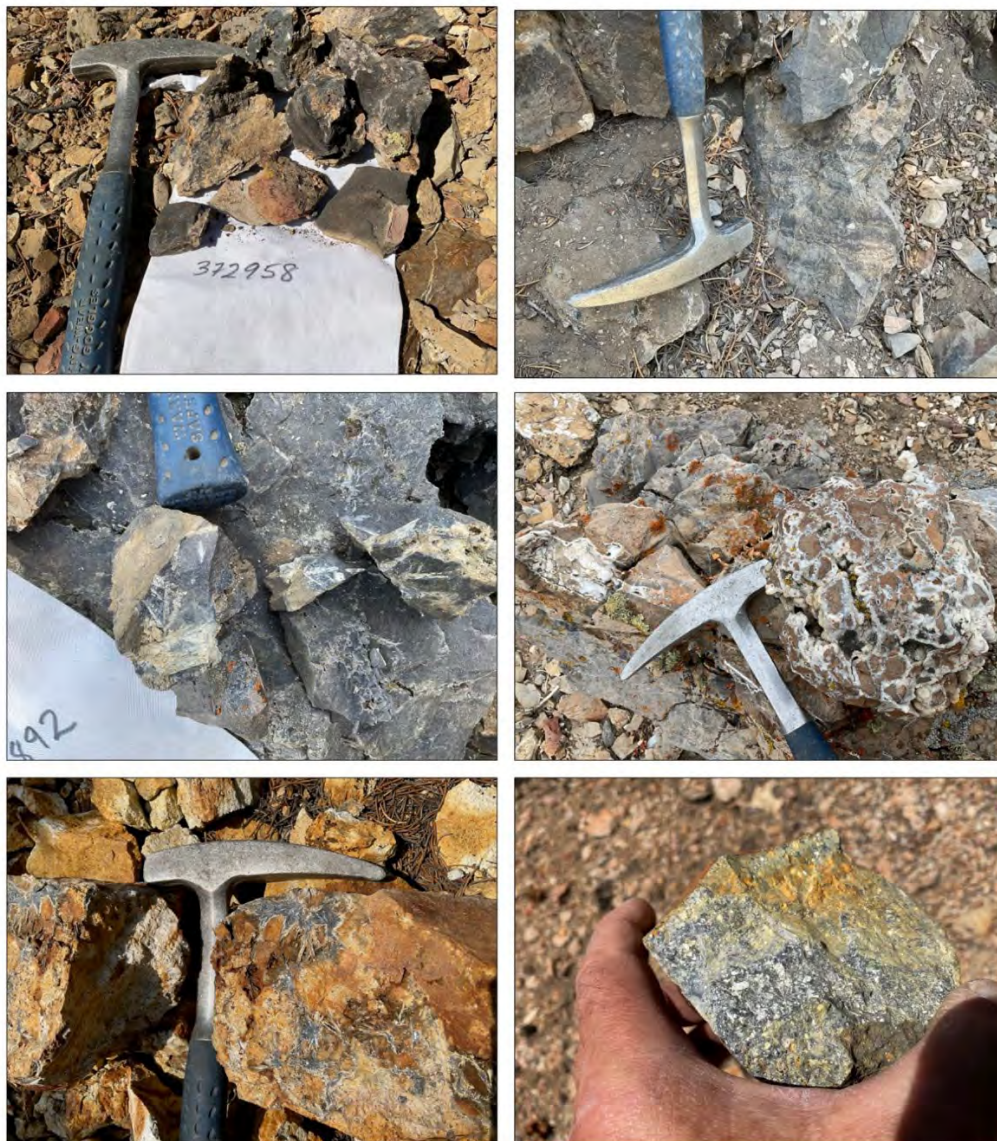
Figure 11. Representative types of mineralization observed at King Solomon. Top left: Decarbonized, porous, carbonaceous silty limestone in the Roberts Mountains Formation (Zn = 1690 ppm); Top right: jasperoid with relict bedding textures in Devonian McColley Canyon Limestone(?) (3.9 g/t Au, 63 g/t Ag); Middle left: jasperoid with late stibnite-stibiconite in voids and fractures, Devonian McColley Canyon (26 ppb Au, 39 g/t Ag, 38 ppm As, >1% Sb, 28 ppm Se); Middle right: Jasperoid of the Roberts Mountains Formation with late-stage white, drusy quartz infilling irregular vugs (165 ppb Au, 266 g/t Ag). Bottom left: Silicified and sericitized House porphyritic rhyolite with late-stage stibnite-quartz-barite in irregular vug infilling (2.82 g/t Au, 609 g/t Ag, >1% Sb); Bottom right: Polymictic rhyolite intrusive breccia from King Solomon antimony mine with fine-grained stibnite (389 ppb Au, 278 g/t Ag, >1% Sb).
